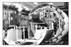
Rulmeca Motorized Pulleys have been incorporated into Tunnel Boring Machines (pictured above) for years. However, they are not "intrinsically safe" or "flame proof" and are not suitable for service where explosive gasses, vapors, liquids, or dust are continuously present. Contact Rulmeca for additional details.
