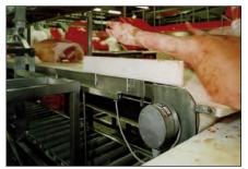
Environments with high amounts oil, grease, and/or fat require special oil-resistant lagging. If they require frequent high pressure and/or chemical cleaning they may also require regreasable seals and stainless steel or special surface coating. See pages 82 and 87.
