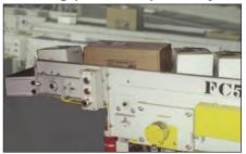
Electromagnetic brake provides excellent product "hold" capability in induction systems requiring "indexing." See page 81.
